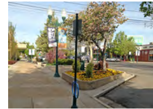
A pedestrian-friendly sidewalk with planted bulb out that shortens pedestrian crossing distances
